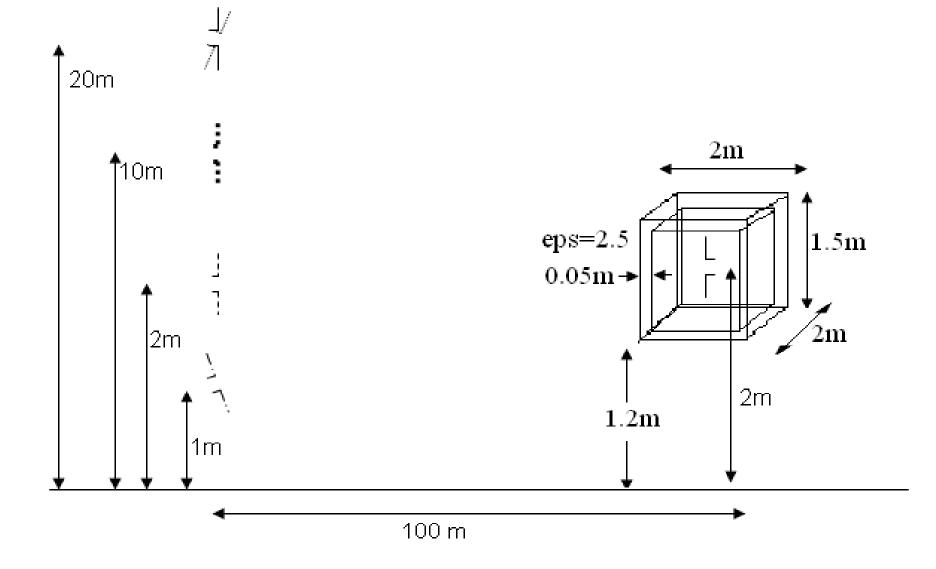
Different transmitting dipole configurations at a height of 20 m, 20 m tilted downwards at an angle of 11°, 10 m, 2 m and 1 m tilted upwards by an angle of 1° above the ground plane. The receiving dipole is located at 2 m above the ground plane and at a horizontal distance of 100 m from the transmitter. The receiving dipole is enclosed by a dielectric shell.
