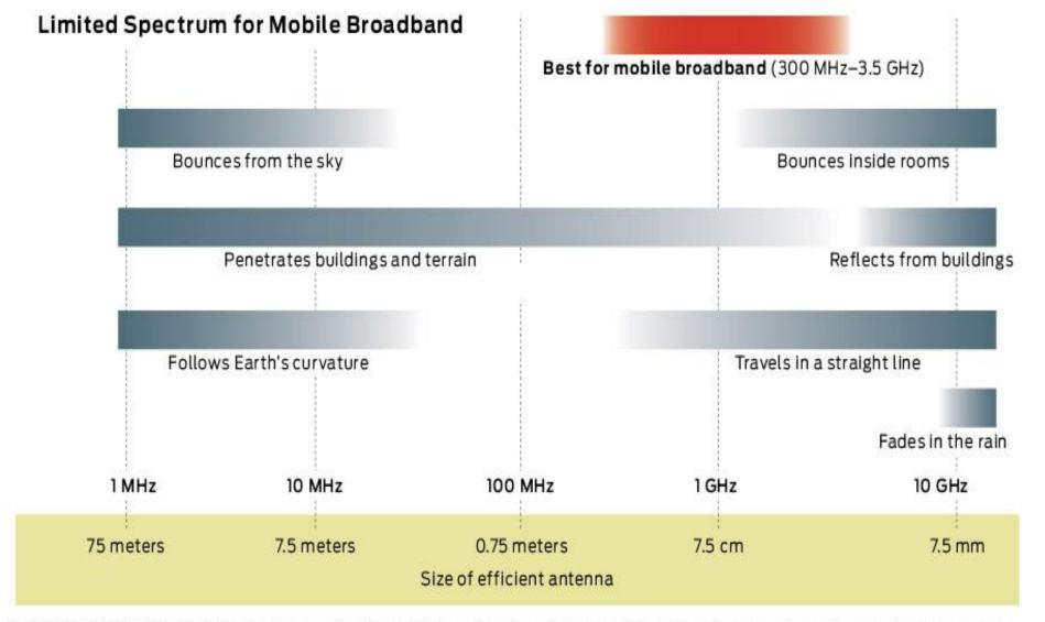
**OPPORTUNITY WINDOW:** The best frequencies for mobile broadband are high enough that the antenna can be made conveniently compact, yet not so high that signals will fail to penetrate buildings. This leaves a relatively narrow range of frequencies available for use [red band].
