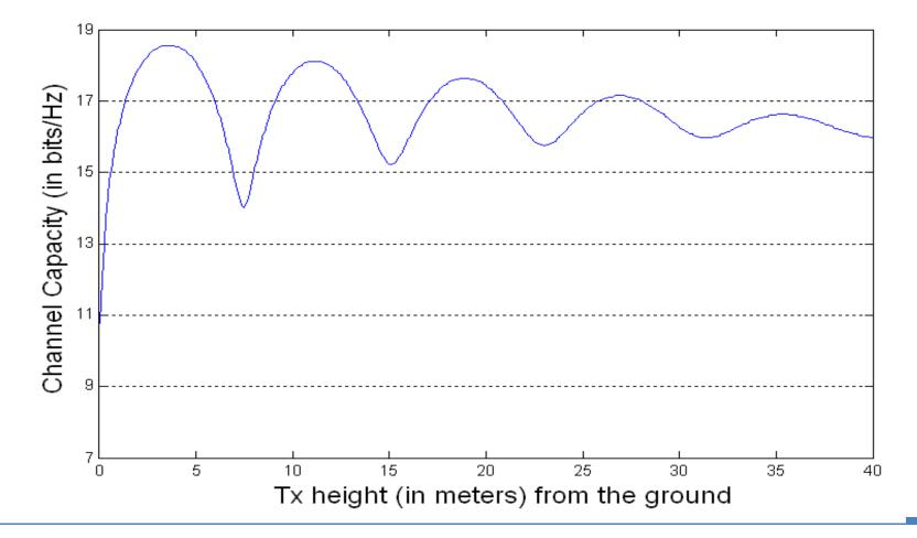
Load on the received antenna (Rx Ant HT = 2M)
