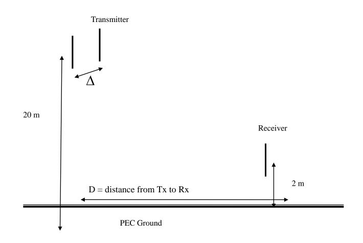
MISO system setup; Transmitter is 20 m. above ground; Rx is 2 m. above ground; = transmitting antenna spacing; D = distance between the transmitter and the receiver. (For the SISO case, the transmitting antenna is placed at the center of the MISO transmitter.)
