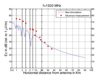
Comparison between Okumura's drive test measurements and the numerical analysis done using Schelkunoff Integrals
