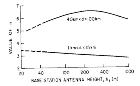
**Figure 2.2-14** Distance dependence of median field strength in an urban area  $P_r \alpha d^{-n}$ ).
