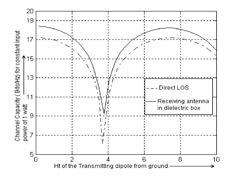
Comparison of the plots of the variation of the channel capacity as a function of the height of the transmitting antenna above a perfectly conducting earth, for a fixed height of 2 m for the receiving antenna. LOS stands for line-of-sight.
