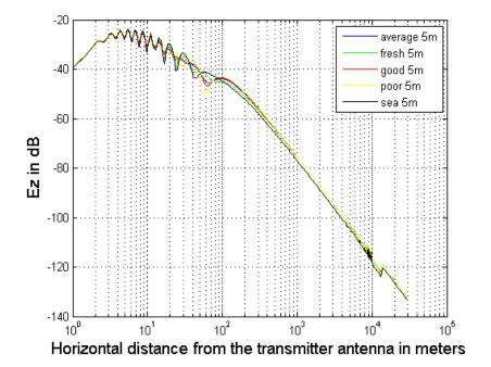
Variation of magnitude of Ez from a half-wavelength dipole as a function of distance, at an operating frequency of 900 MHz. The height of the observation point was 2 m. Five different types of ground have been used, with different parameters.
