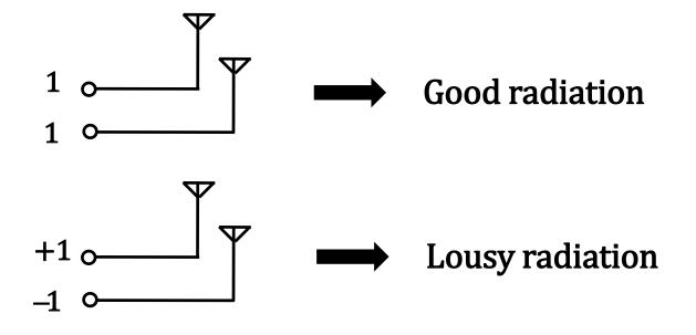
Hence, even though simultaneous multiple channels are possible, only one is practical and the others are not very useful from a systems perspective
