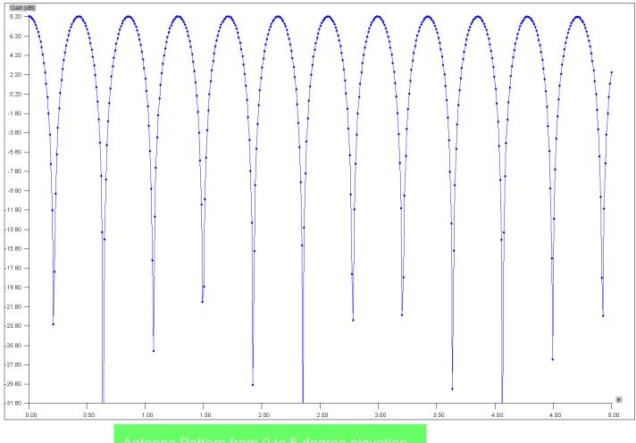
Antenna Pattern from 0 to 5 degree elevation
