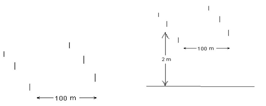
A typical  $3 \times 3$  MIMO system consisting of half wave dipoles, half wavelength spaced and separated by 100 m.
