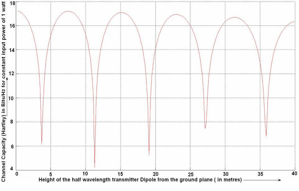
Plot of the variation of the channel capacity as a function of the height of the transmitting antenna above a perfectly conducting earth, for a fixed height of 2 m for the receiving antenna.
