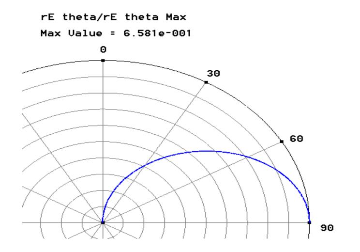
The radiation pattern of a half wave dipole in free space (only one fourth shown)
