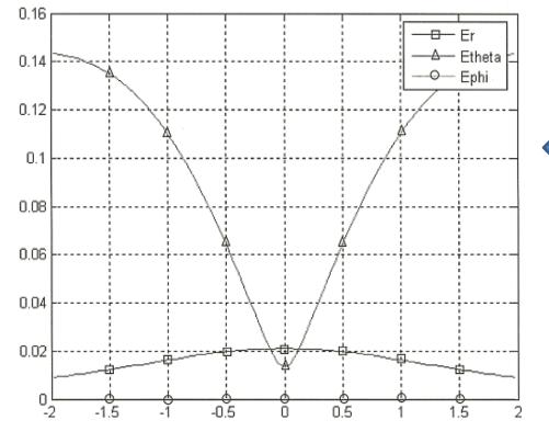
The three components of the fields *Er*, *E* $\theta$ , *E* $\phi$  inside the room at x = -0.0198\lambda, z = -3.75 $\lambda$ , as a function of y
