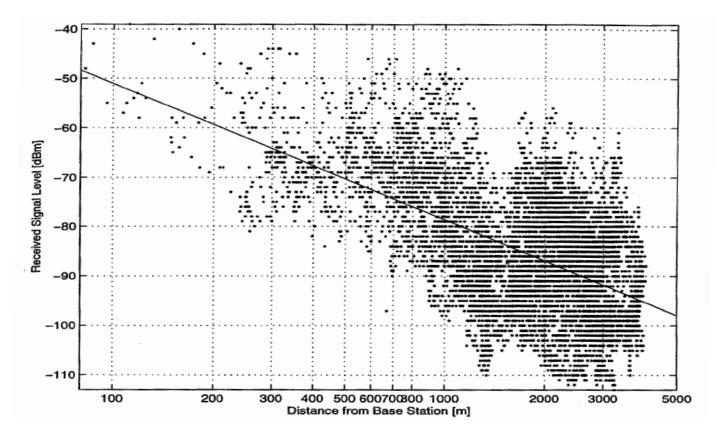
Empirical model of macrocell propagation at 900 MHz, the dots are measurements taken in suburban area, where as the solid line represents a best fit empirical model. Reproduced by permission from Simon R. Saunders, Advances in mobile propagation prediction methods, Chapter 3 of *Mobile Antenna Systems Handbook, Third edition*, Edited by: Kyohei Fujimoto, 2008, Artech House, Inc.
