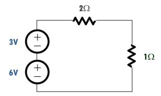
Applied Superposition Power Dissipated in  $1\Omega$ =  $I^2 R = 3^2 \cdot 1 = 9$
