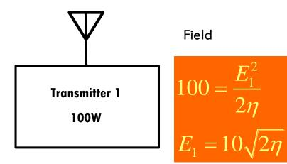
Interference occur between the fields *E1* and *E2*. So the variation in field is
