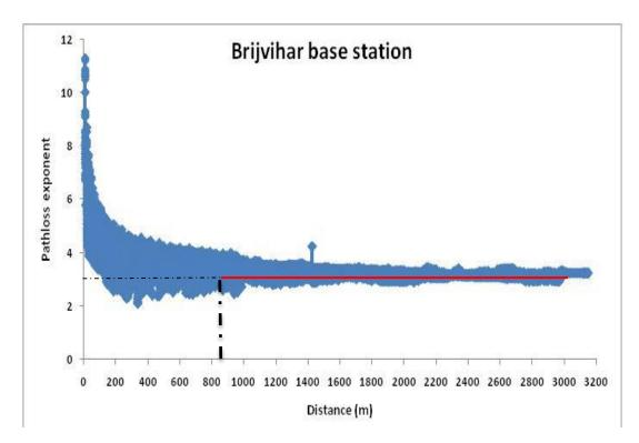
Variation of path loss exponent with distance for BJV base station (1800 MHz). Base station height: 24 m. Beginning of smooth region: 864 m.
